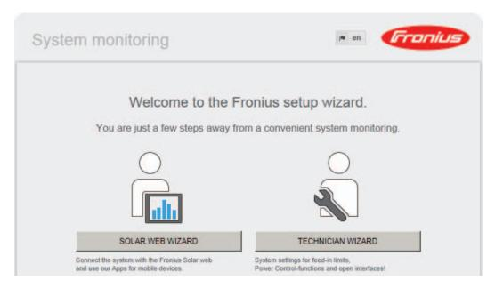
If you run the technician wizard, always remember to make a note of the assigned service password. This service password is necessary for making settings in the "System overview" and "EVU Editor" [UC Editor] menus as well as for advanced battery settings. If the technician wizard is not run, no specifications regarding power reduction are set and hybrid mode is not possible (charging and discharging of the Fronius Solar Battery).
