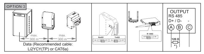
\*) The R 120 Ohm terminating resistor is included with the Fronius Smart Meter
