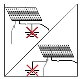
The Hybrid inverter is a transformerless device. The individual poles of the solar modules must not be grounded.
