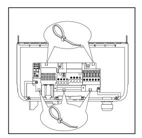
If overlength AC or DC cables are to be laid in loops in the connection area, attach the cables with cable ties to the eyelets provided on the top and bottom of the connection block.
