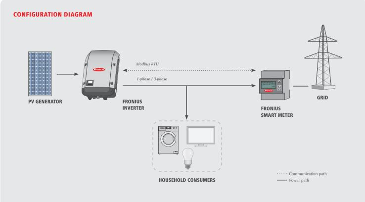
/ The Fronius Smart Meter is compatible with all inverters with an RS485 interface (Modbus RTU). The Fronius Smart Meter works in conjunction with the Fronius Datamanager 2.0 for the Fronius IG Plus inverters, whereas the Fronius Datamanager Box 2.0 is used with the Fronius Agilo inverter. The Fronius Smart Meter can be retrofitted at any time together with the Fronius Datamanager 2.0 in inverters that have already been installed.
