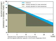
At least 97 % of nominal power during first year. Thereafter max. 0.6 % degradation per year. At least 92 % of nominal power after 10 years. At least 83 % of nominal power after 25 years. All data within measurement tolerances.
