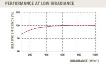
Typical module performance under low irradiance conditions in comparison to STC conditions (25°C, 1000W/m<sup>2</sup>).
